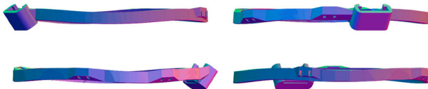
Fig. 2. Improved frame model in color lighting on four sides for better visibility of added curvatures and final shape
